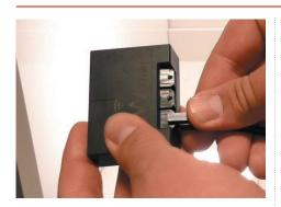
Plug either cable into the left-hand side of the control module
