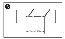
Using the mounting template mark the desired location for installation.
