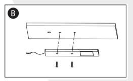
2 Fix the mounting screws to the two positions marked in the desired location.
