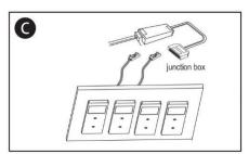
Connect the fittings to the junction box on the driver.
