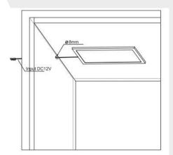
Thread the connector through a 2 hole to the LED driver.
