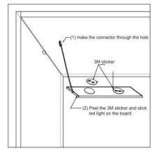
Create a 8mm diameter hole for the connector cable to reach the LED driver.
