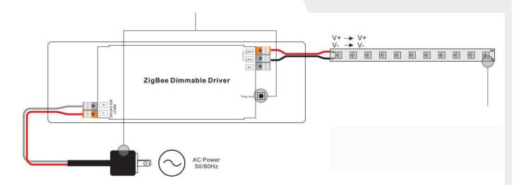
Connected light will blink 3 times to indicate successful reset
