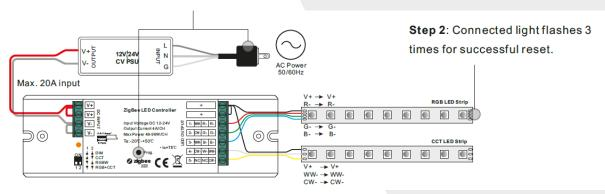
Note: 1) If the device is already at factory default setting, there is no indication when factory reset again. 2) All configuration parameters will be reset after the device is reset or removed from the network.
