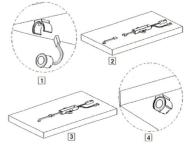
2. Installation way two: open cable channel on the wood panel as figure picture, fix related length of cable channel base, plug the sensor switch cords through the hole of back board. Then fix sensor switch, install the cover board of the cable channels.
